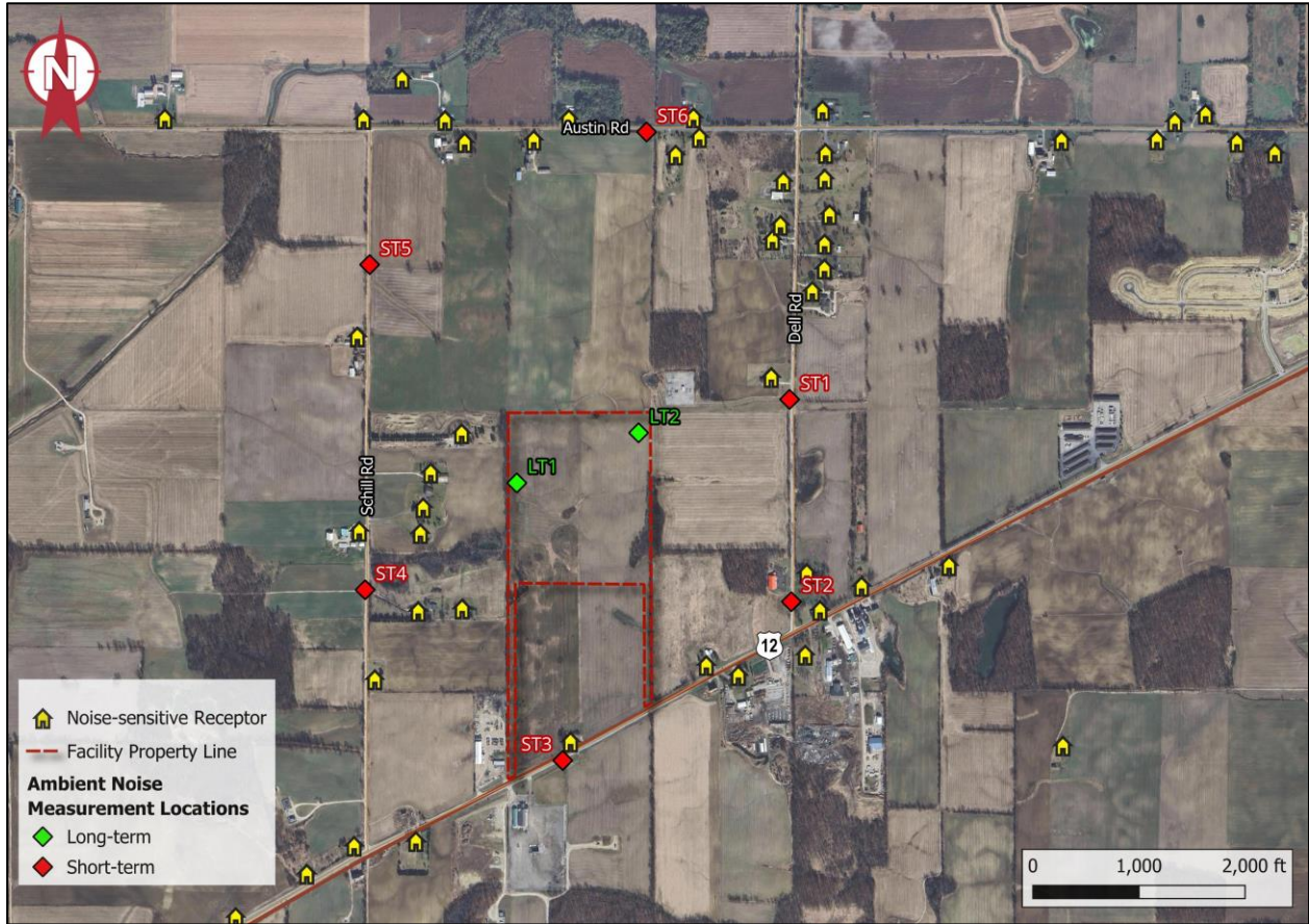
Figure 3-1. Ambient Noise Measurement Locations
